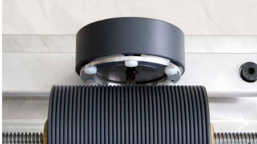
Figure 8: During assembly, the mandrel is positioned on the threaded rod so that the stylus is centered in the groove of the mandrel.
