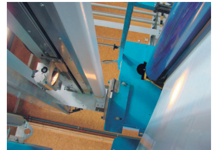
Fig. 1: Reflection sensor head installed in a continuous production line.
