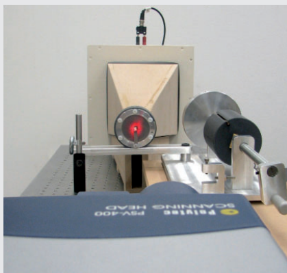
Fig. 4: Photograph of the measurement apparatus for diaphragm velocity.
