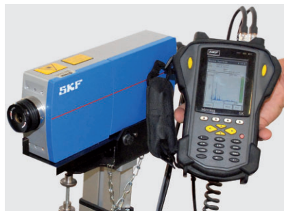
Fig. 3: Mobile vibration analysis kit with SKF laser vibrometer and SKF Microlog.
