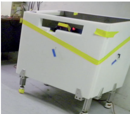
Fig. 3: RSV laser enclosure without lid for shielding of equipment from radiation.
