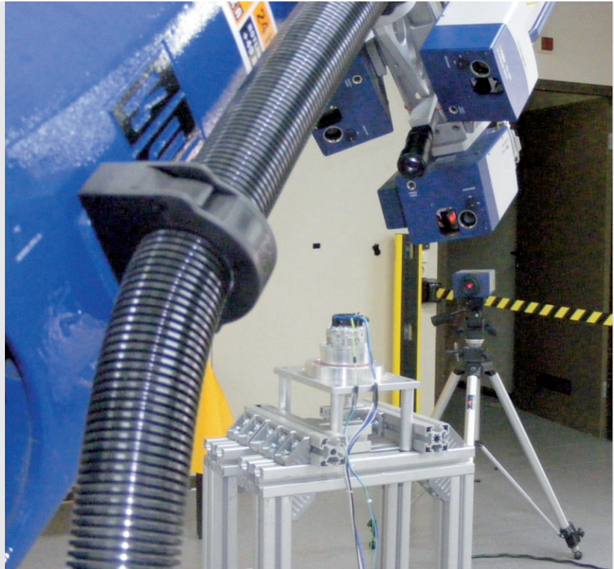
Fig. 4: Vibration measurement on a vacuum cleaner motor.
